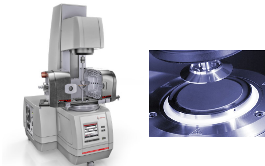
Figure 4.2: Anton Paar rheometer of type MCR102 with additional a temperature chamber (left) and the plate-plate measuring geometry (right)
