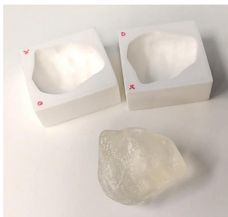
Figure 7: Example of 3D printed lung equivalent boxes, with hydrogel tumor.
