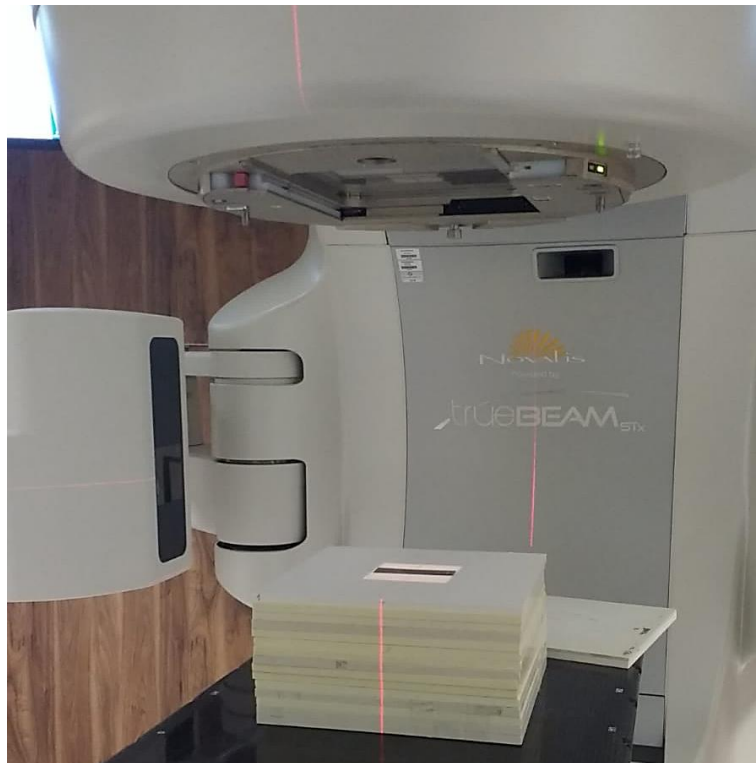
Figure 11: Set up of film calibration with the TrueBeam linac at Jessa Hospital.
