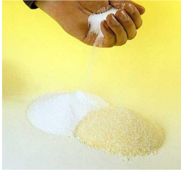
Figure 10: Raw candle material made by means of spraying drums [4]
