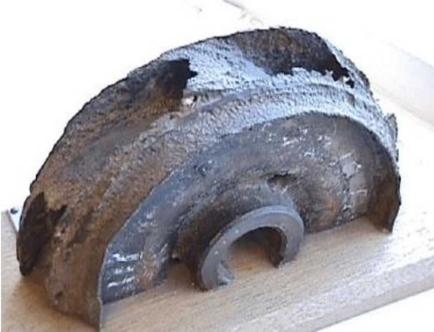
Figure 63: Damage by cavitation in centrifugal pump [52]
