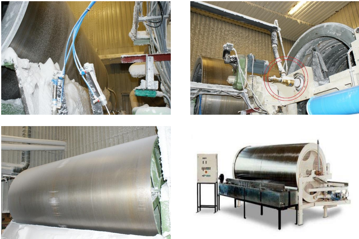
Figure 9: Pulverization of liquid raw candle material by means of spraying drums at Suomen Kerta [4]
