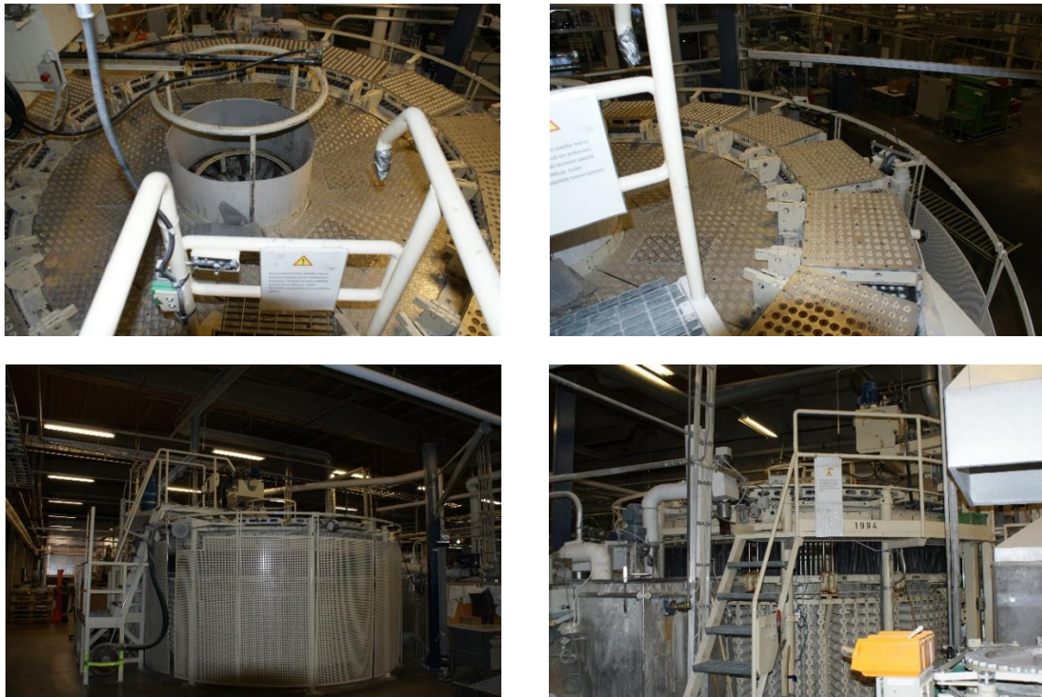
Figure 7: Machine a: rotary molding machine used at Suomen Kerta factory
