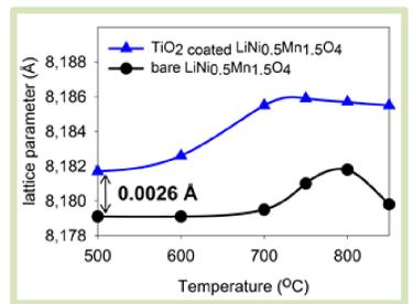
Refined lattice parameters of LNMO@TiO<sub>2</sub> are slightly higher than that of bare LNMO
