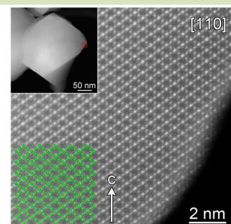
Well preserved spinel surface structure of LNMO@TiO<sub>2</sub> upon 800°C anneal
