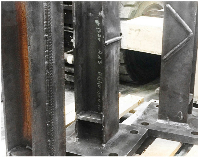
Fig. 5. Applied shear connectors – a view on the welded connectors.
