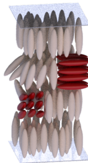
Figure 9. Sketch of the molecular structure of confined 8CB. The functionalized solid surfaces (blue) induce an orientation with the LC director parallel to the interface normal (brown). Grain boundary energies make misaligned domains (red) energetically unstable. However, they can gradually adjust in height during slit-pore opening. During compression, these 8CB dimers get integrated into the majority domain (brown), leading to an overall increase in alignment.
