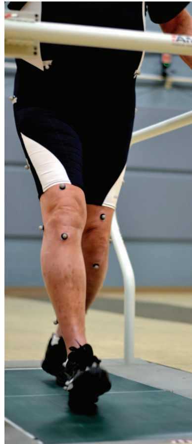
Fig. 1. Gait assessment setup. Infrared cameras are placed throughout the laboratory. Calibrated cameras triangulate the position of each marker based on the reflection of infrared light back to the camera lens off the retroreflective marker. The positions of markers were used to calculate joint angles and range of motion of the joints.
