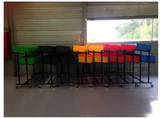
Figure 5: Coloured baskets to indicate the stage in the production process
