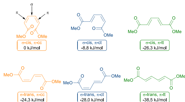
Fig. 5 - The six possible isomers of dimethyl muconates (DMM) and their computed enthalpies relative to \sigma -cis, \pi -cc DMM. \sigma refers to the C3-C4 single bond, while \pi refers to both C2=C3 and C4=C5 double bonds.
