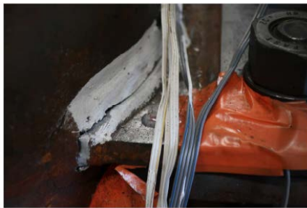
Fig. 15. LASTEICON_LC2 Failure: (a) CHS column wall tearing at the flange plate-to-column connection zone observed from the experiments and (b) Von mises equivalent plastic strains concentrated at the CHS-to-flange connection zone obtained from the numerical model
