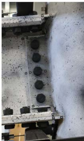
Fig. 16. Conventional_LC1 Failure: (a) CHS chord crushing observed from experiments and (b) Von mises equivalent plastic strains obtained from the numerical model
