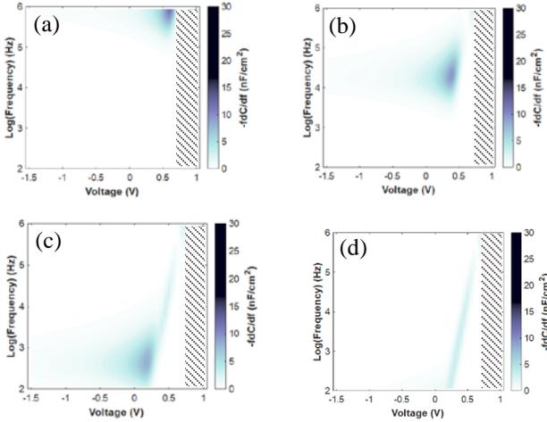
Fig. 8. Simulated loss map of the solar cell device with a donor-type bulk defect of  $10^{16}$  cm<sup>-3</sup> density at an energy position of 0.3 eV (a), 0.4 eV (b), 0.5 eV (c) and 0.6 eV (d) below the conduction band edge energy of the CIGS.
