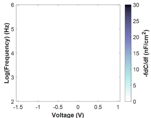
Fig. 5. Simulated loss map of the ideal heterojunction device:  $-fdC/df$  contour plot of the CIGS solar cell device without added defects as a function of DC bias voltage and the logarithm with base 10 of the frequency.
