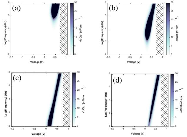
Fig. 9. Simulated loss map of the solar cell device with an acceptor-type interface defect at the CIGS-CdS interface with a density of  $10^{12}$  cm<sup>-2</sup> eV<sup>-1</sup> and at an energy position of 0.3 eV (a), 0.4 eV (b), 0.5 eV (c) and 0.6 eV (d) above the top of the valence band edge energy of the CIGS.
