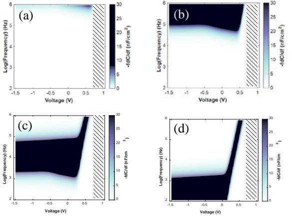
Fig. 10. Simulated loss map of the solar cell device with an acceptor-type interface defect at the CIGS-CdS interface with a density of  $5 \cdot 10^{12} \text{ cm}^{-2} \text{ eV}^{-1}$  and at an energy position of 0.3 eV (a), 0.4 eV (b), 0.5 eV (c) and 0.6 eV (d) above the top of the valence band edge energy of the CIGS.
