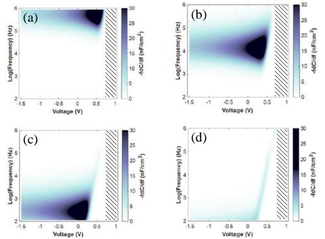
Fig. 7. Simulated loss map of the solar cell device with an acceptor-like bulk defect of  $10^{16} \text{ cm}^{-3}$  density at an energy position of 0.3 eV (a), 0.4 eV (b), 0.5 eV (c) and 0.6 eV (d) above the valence band edge energy of the CIGS.
