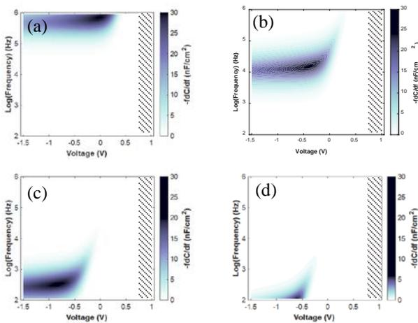
Fig. 11. Simulated loss map of the solar cell device with low CdS doping of about  $10^{17} \text{ cm}^{-3}$  and with a donor-type interface defect at the CIGS-CdS interface with a density of  $10^{12} \text{ cm}^{-2} \text{ eV}^{-1}$  and at an energy position of 0.3 eV (a), 0.4 eV (b), 0.5 eV (c) and 0.6 eV (d) below the bottom of the conduction band edge energy of the CIGS.
