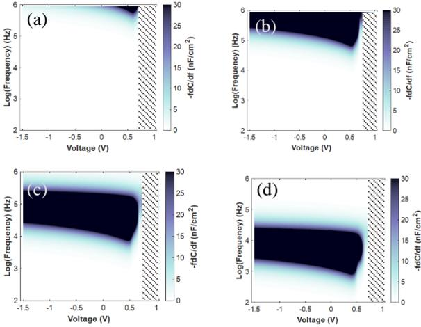
Fig. 6. Simulated loss map of the solar cell device with a series resistance of  $1 \Omega \text{ cm}^2$  (a),  $10 \Omega \text{ cm}^2$  (b),  $100 \Omega \text{ cm}^2$  (c) and  $1000 \Omega \text{ cm}^2$  (d). The grey hashed-out area highlights the forward bias region where the junction capacitance collapses, and the simulation results are not reliable.
