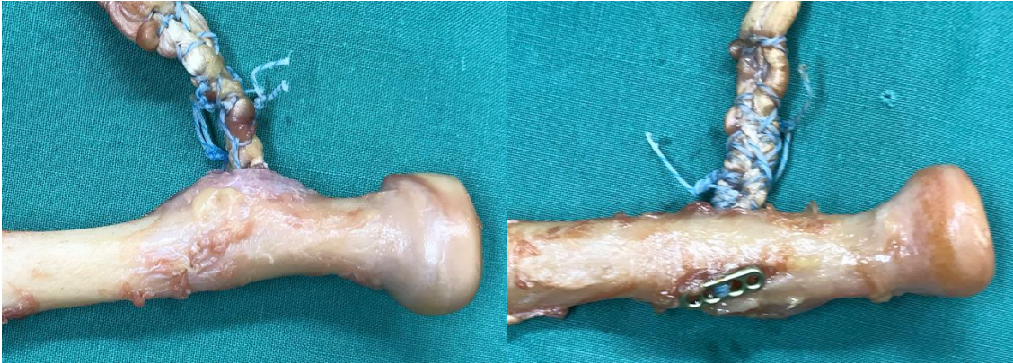
Figure 3 (a and b): The two different setups showing one with an intramedullary and one with an bicortical fixation.
