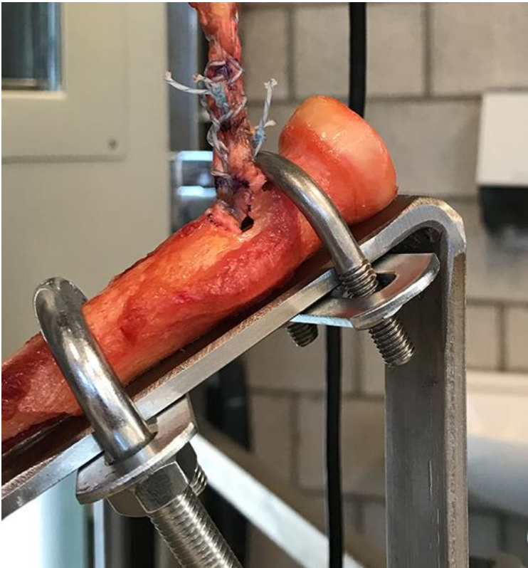
Figure 4: The test setup with a custom mount at 30° to simulate the native line of pull. Hand drawn lines were used for measurement of displacement.
