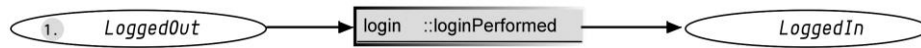
Fig. 4. Excerpt from the Petri net model of the standard behavior of the application: event handling of the login action. In the transition, the text on the left describes the name of the transition while the text on the right describes the name of the event associated the transition.
