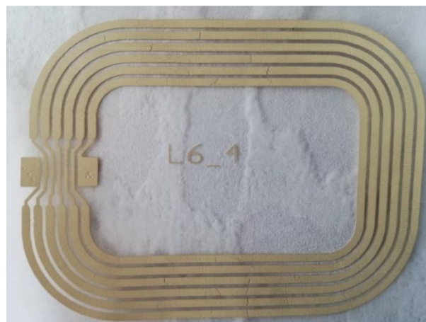
Figure 50: Crack formation on conductive paths; Orgacon ink on TPU1
