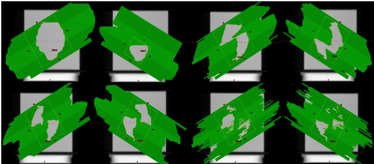
Figure 8 MLC positions at the same angle in the arc for four plans with different amounts of complexity of the same patient. Top left: no modulation, top right: low modulation, bottom left: medium modulation, bottom right: high modulation.
