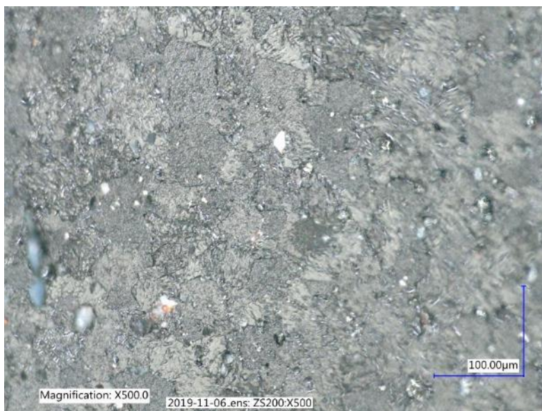
Figure 16: Damage resulting from the piranha etch
