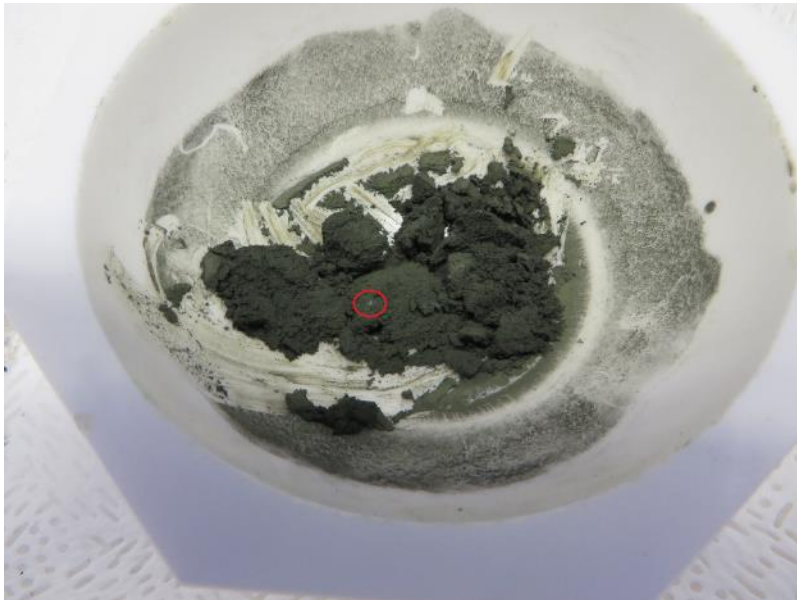
Figure 13: Image of inhomogeneities present in the ADU batch. Presumed to be \text{Cr}_2\text{O}_3 .
