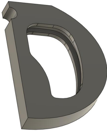
Figure 18: Designing of a 3D-volume for the thorax phantom showing the design of one rib on one side
