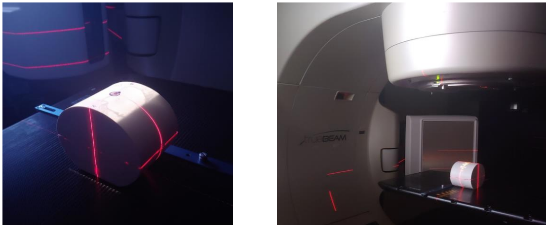
Figure 15: Positioning of the thorax phantom in the linac with visible reference points
