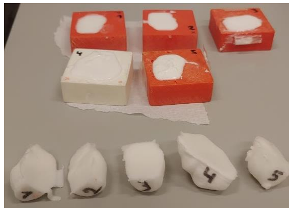
Figure 11: Samples of silicone mixed with CaCO 3 with five samples curing in 3D-printed tumor molds
