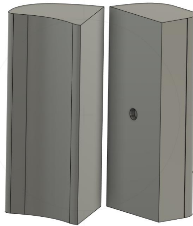
Figure 24: Design of two part right lung containing 1 alanine insert
