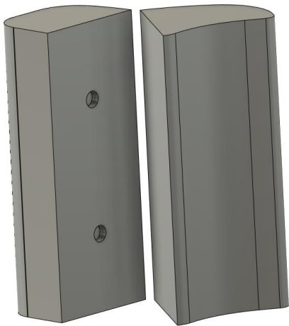
Figure 23: Design of two part left lung containing 2 alanine inserts
