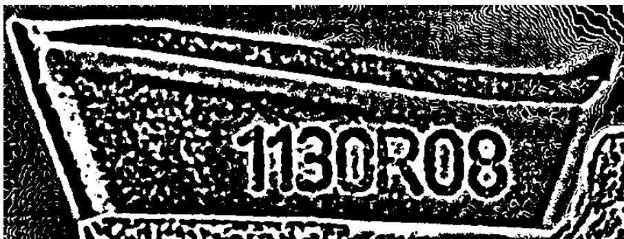
Figuur 54: Laplace filter na adaptive thresholding met kernel = 501
