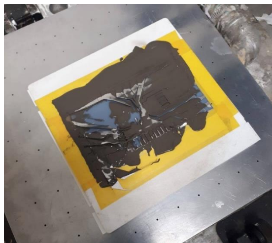
Figure 6.13: Substrate and mask after passing of squeegee
