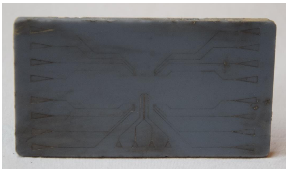
Figure 6.14: 3D printed substrate after screen printing and cleaning
