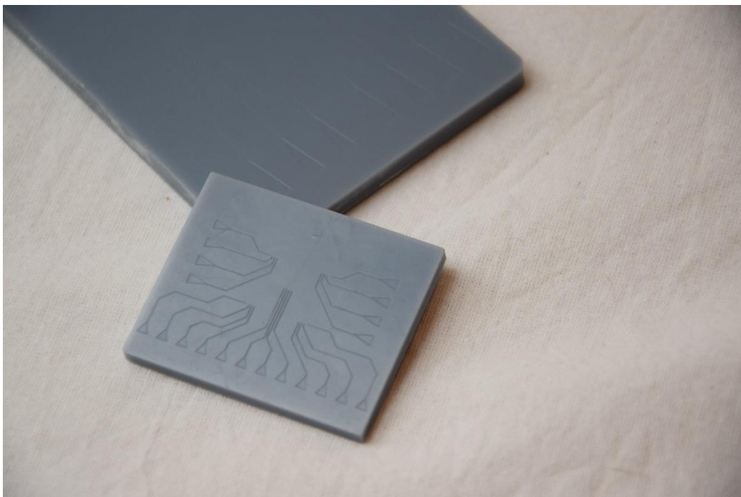
Figure 6.11: Top probe 3D printed substrate
