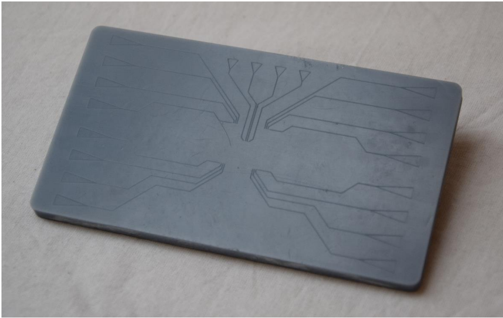
Figure 6.10: Bottom probe 3D printed substrate
