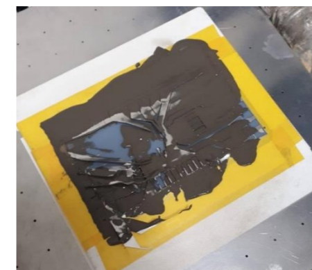
Broken printing mask
