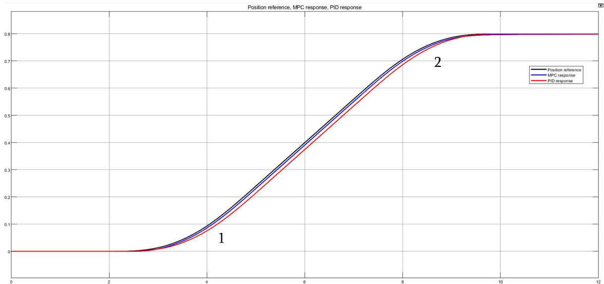
Figure 54: Comparison of MPC response and PID response with belt position as measured variable
