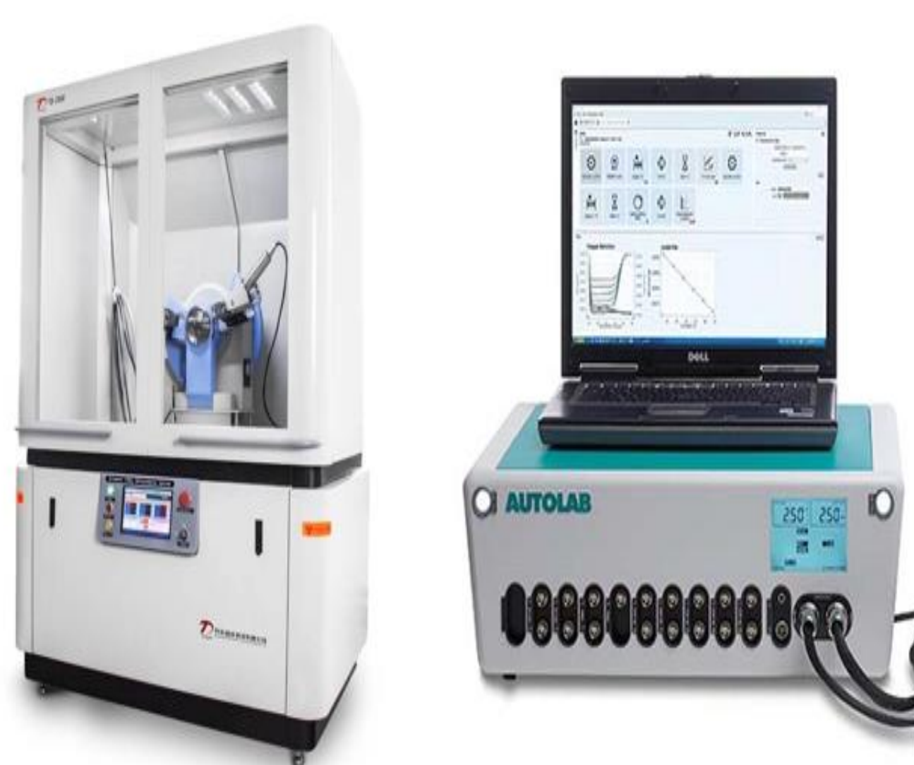
Figure 2. XRD-apparatus (left) and an Autolab to execute cyclic voltammetry and electrochemical impedance spectroscopy (right)
