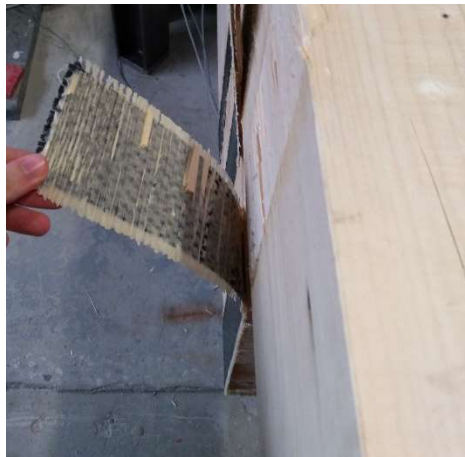
Figure 38 Surface of debonded reinforcement after failure
