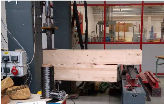
Figure 36 Shear crack after failure of the unreinforced beam
