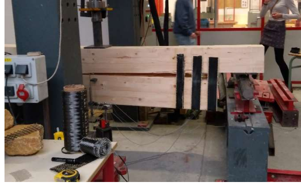
Figure 37 Shear crack after failure of the reinforced beam
