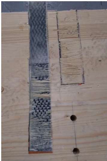
Figure 29 L200_45_d shows a typical failure mode, with a combination of failure in resin and timber surface
