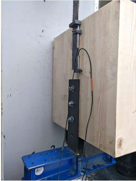
Figure 16 Placement of LVDTs during single lap shear tests
