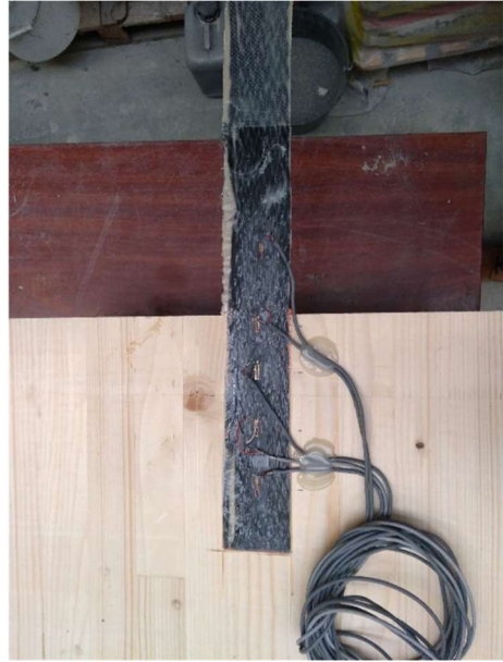
Figure 17 Placement of strain gauges during single lap shear tests
