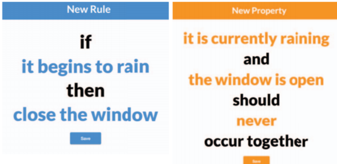
Figure 2.10: AutoTap: On the left: a (buggy) trigger-action rule.; On the right: a proposed trigger-action property. The trigger-action rule (left) cannot guarantee the property (right) [58].
