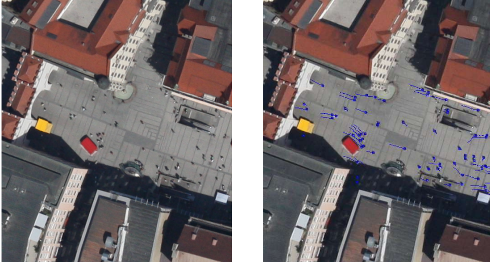
Figure 4.1: Frame of KIT dataset for tracking people in aerial image sequences, with on the left pre labeling and on the right post labeling [70]
