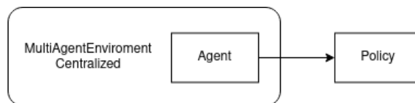
Figure 4.7: Illustration of multi-agent case that uses a centralized approach
