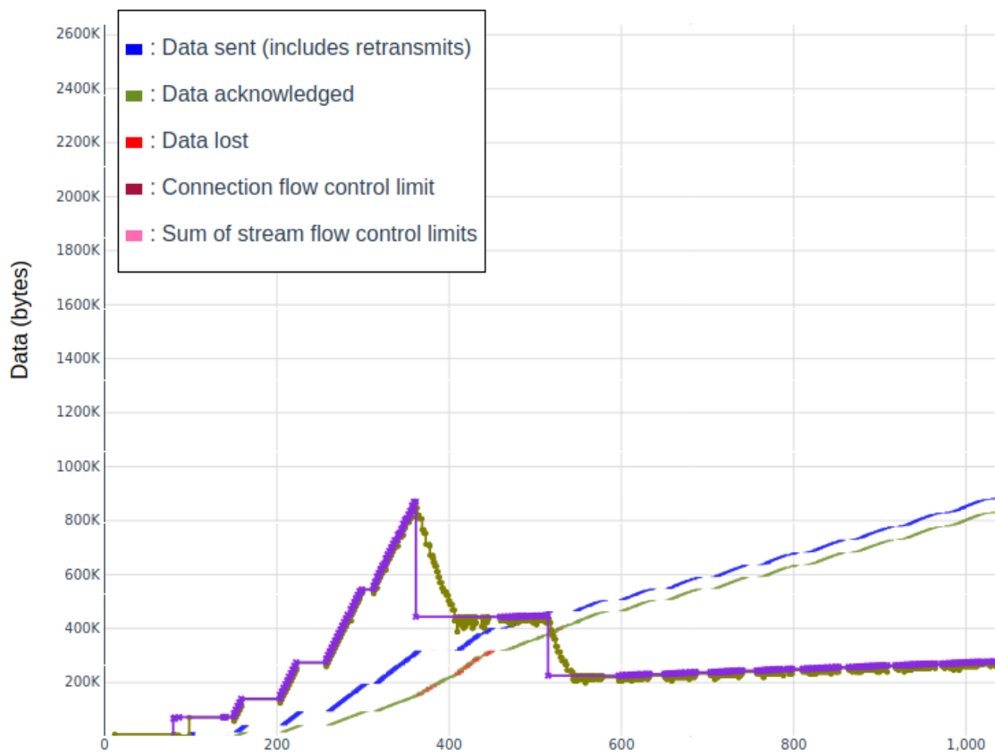
Figure 36: Quant’s two shorter recovery periods in interval of 1 second in NS-3, CWND as purple line
