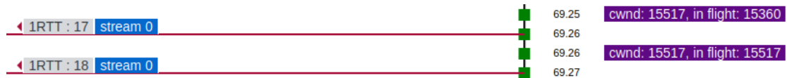
Figure 27: qvis sequence diagram showing the second packet only increasing the bytes in-flight by smaller value in Aioquic
