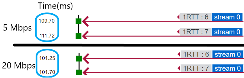
Figure 22: Time difference between two packets arriving with two different bandwidths in NS-3
