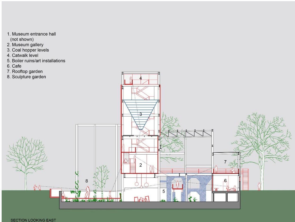
FIGURE 65 SECTION LOOKING EAST WITH PROGRAM AND CONNECTING VIEWS IN THE BUILDING (SHOWN IN DASHED LINE)
