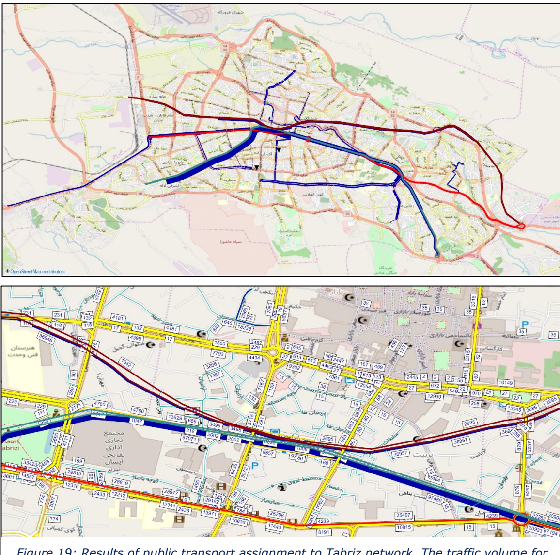
Figure 19: Results of public transport assignment to Tabriz network. The traffic volume for each road is written beside it. (Blue line: The number of passengers using a certain link. The thickness of the line is a function of the number of passengers. Turquoise line: Metro line 1. Dark red line: Metro line 2. Light red line: BRT.) (Source: Created by the author in PTV Visum in January 2020)
