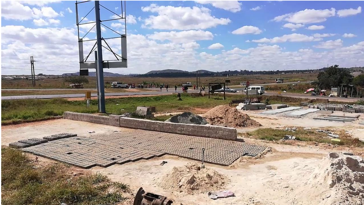
Figure 19: Brick Moulding site in the open space besides the Junction source: Self, 2020
