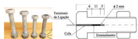
b) Strain gauges inside the bolts
