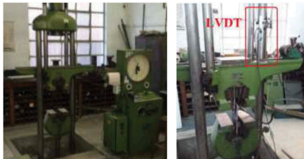
Figure 2. Universal machine and LVDT position used in experimental tests.
