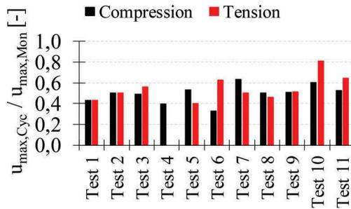
Figure 6. Comparison between the maximum deformation of the U-Shape steel plate connection under cyclic (ECCS cyclic loading protocol) and monotonic loading.
