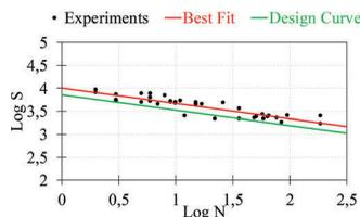
Figure 8. Best fit and low cycle fatigue design curves.
