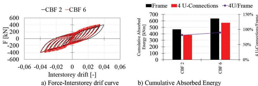
Figure 5. Results of the experimental tests on CBFs incorporating U-Shaped steel plate connection (CBF2 vs CBF6).
