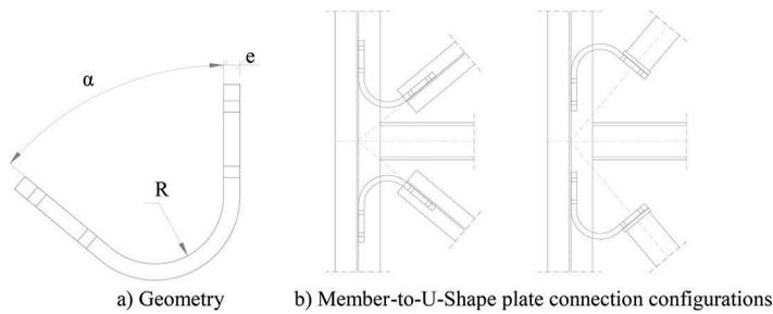
Figure 1. U-shape steel plate connection and its application.
