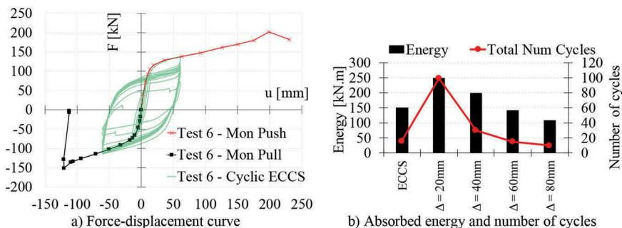
Figure 3. Results of the experimental tests on isolated U-Shaped steel connection.
