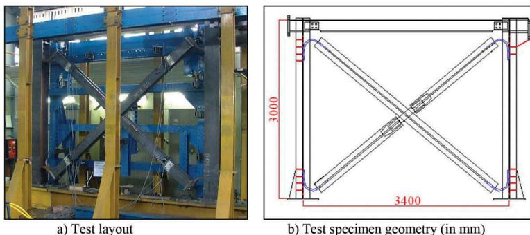
Figure 4. Experimental tests on CBFs incorporating U-Shaped steel plate connection.
