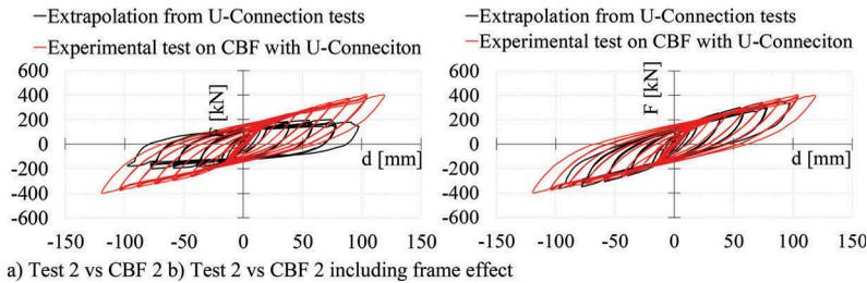
Figure 7. U-Shape steel plate response vs CBF response.
