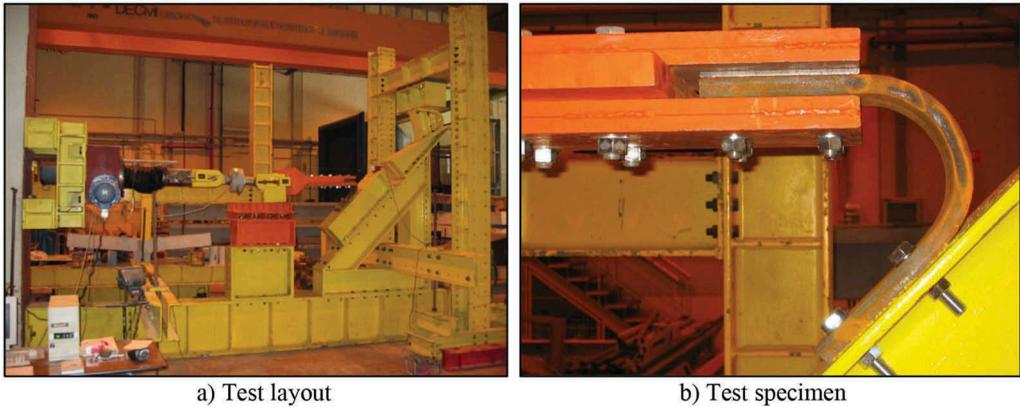
Figure 2. Experimental tests on isolated U-shaped connection (Plumier, A. et al, 2004).
