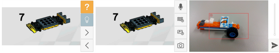
Fig. 1. Left: the assembly instructions are shown with a minimal navigation interface that allows to go to the next/previous step, give feedback on the current step, and get additional help. Middle: The feedback menu allows to record audio, to flag an unclear description or an unclear picture, and to activate the camera with zoom (right).
