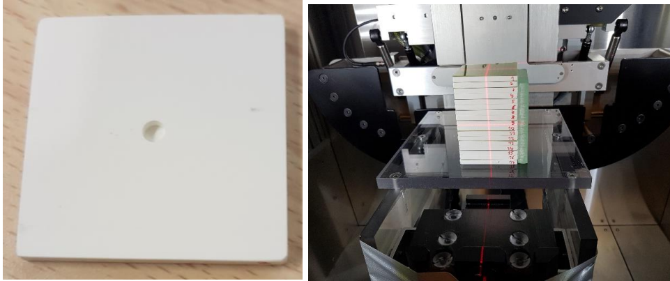
Figure 2-5: Left: 1 slab of the RW3 phantom containing the hole for the alanine detector. Right: a stack of 14 RW3 slabs containing film and alanine detectors.
