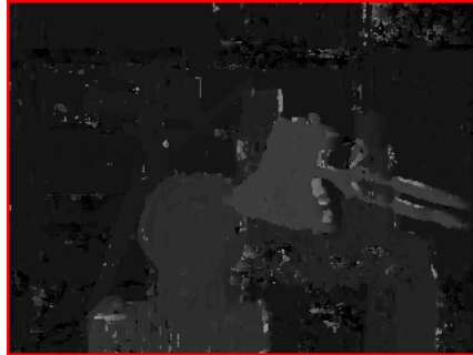
Figure 3.6: Disparity map for the left image of the Tsukuba data set, computed by a local stereo depth estimation algorithm. Red pixels represent pixels that are not assigned a depth value
