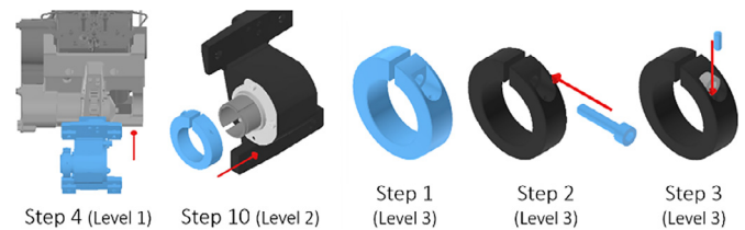
Fig. 4. Visualization of the work instructions for a Picanol weaving machine. Illustrates the sequential actions on different levels of the assembly. Same use-case as in Fig. 5.
