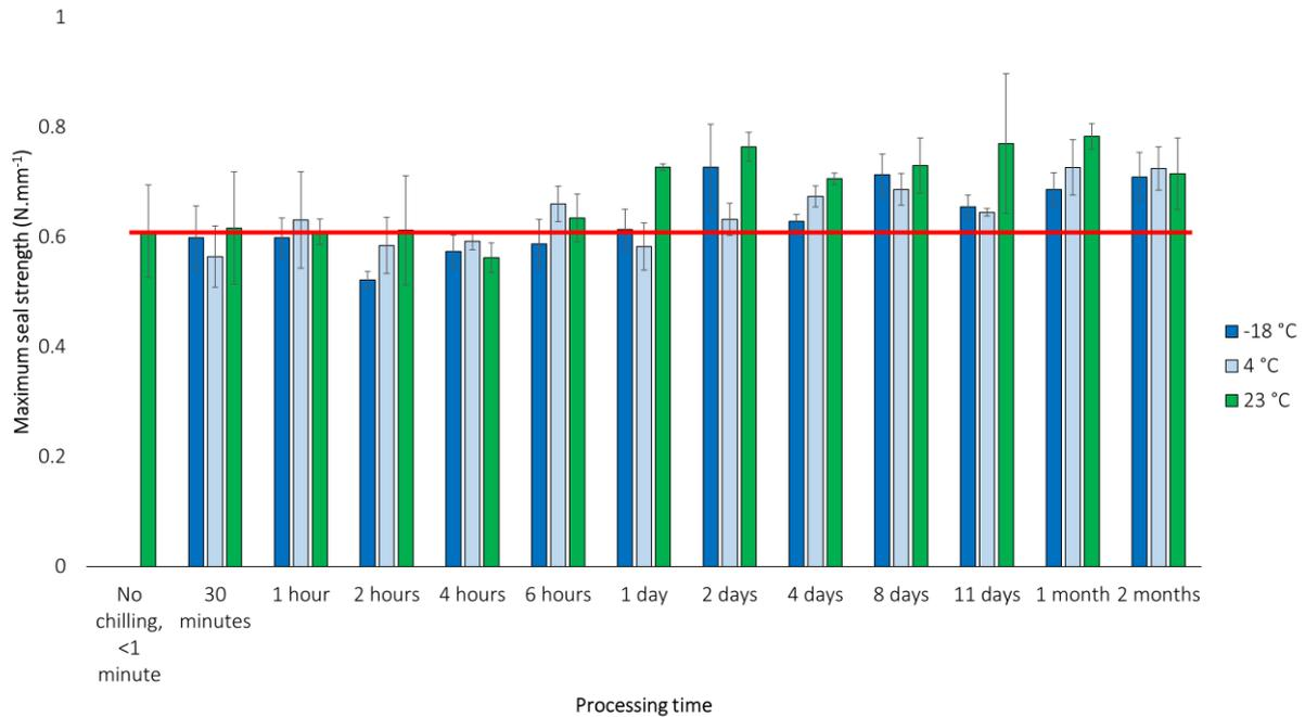
**Figure 3: Influence of processing time on maximum seal strength of PET/PE-EVOH-PE peel 12/45 topfilm, sealed to PET/PE 250/35 non-peel bottomweb, n=3: average value and standard deviation**
