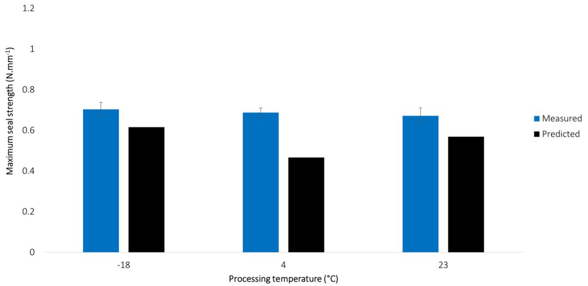
**Figure 14: Experimental validation of optimal maximum seal strength after processing of PET/PE-EVOH-PE (peel) 12/45, sealed against a PET/PE bottomweb**
