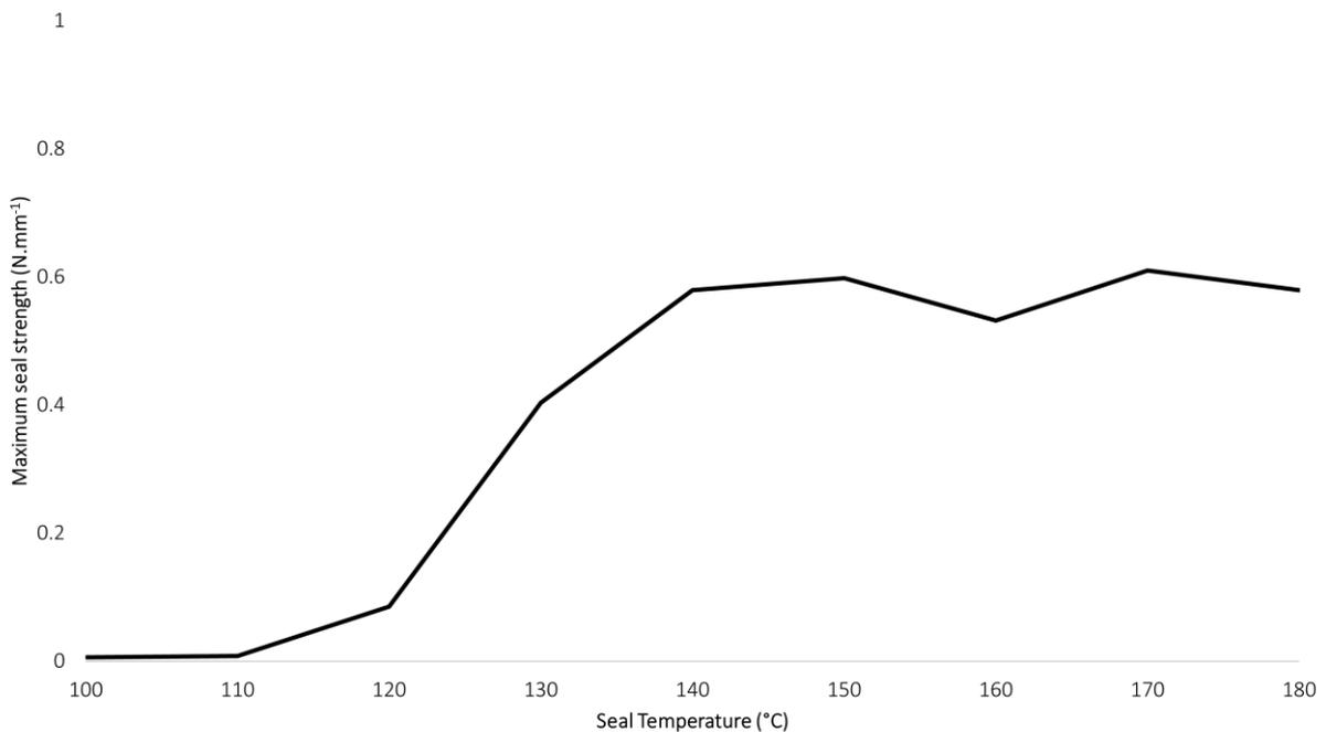
**Figure 10: Influence of upper jaw temperature on maximum seal strength of PET/PE-EVOH-PE (peel) 12/45, sealed against a PET/PE 250/35 bottomweb**
