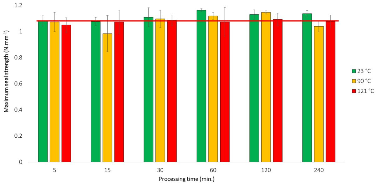
**Figure 4: Influence of processing time on maximum seal strength of PET/PP peel 12/45 pouch, n=3: average value and standard deviation**
