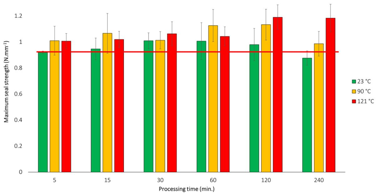
**Figure 5: Influence of processing time on maximum seal strength of PET/PP peel 12/45 topfilm, sealed to PA/PP 60/100 non-peel bottomweb, n=3: average value and standard deviation**
