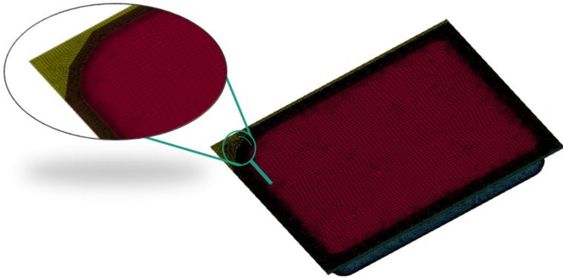
**Figure 7: Meshed geometry model of the package with a locally finer element size in the area of the sealed seal**
