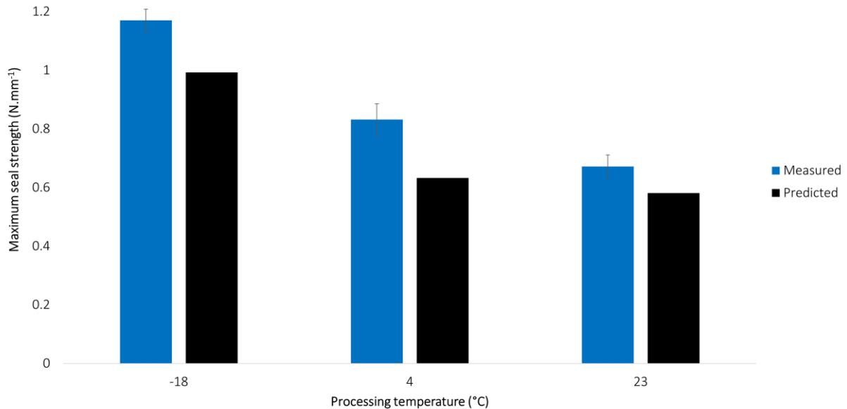
**Figure 13: Experimental validation of optimal maximum seal strength during processing of PET/PE-EVOH-PE (peel) 12/45, sealed against a PET/PE bottomweb**
