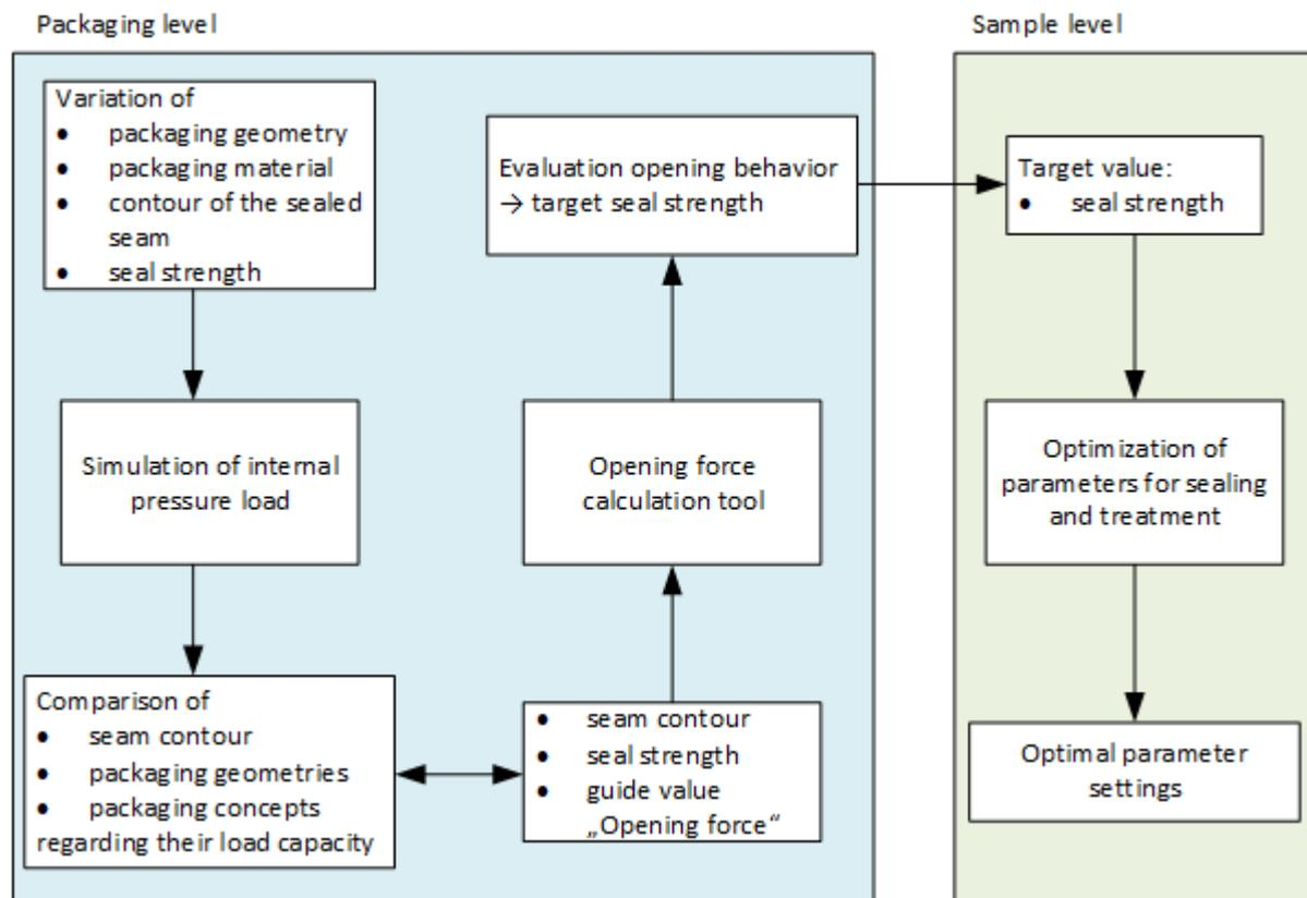
**Figure 23: Guideline to evaluate and optimize peelable packaging concepts undergoing thermal processing**
