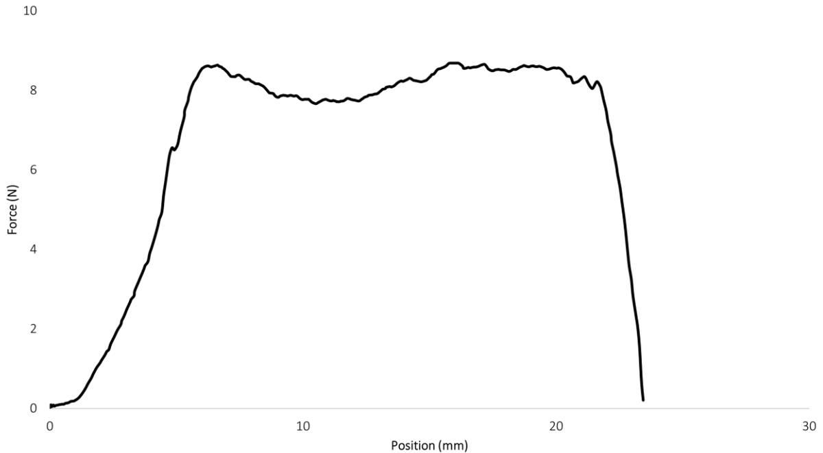
**Figure 9: Raw seal strength curve of peeled PET/PE-EVOH-PE (peel) 12/45 topfilm, sealed against a PET/PE 250/35 bottomweb**
