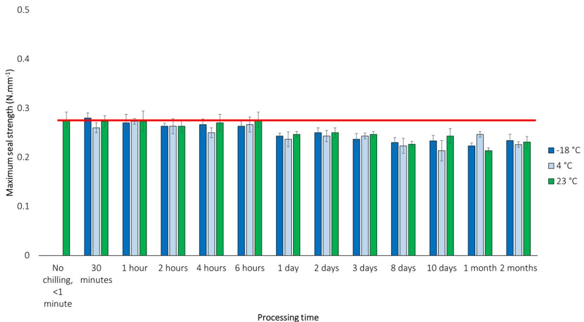
**Figure 2: Influence of processing time on maximum seal strength of PET/PE-EVOH-PE peel 12/45 pouch, n=3: average value and standard deviation**
