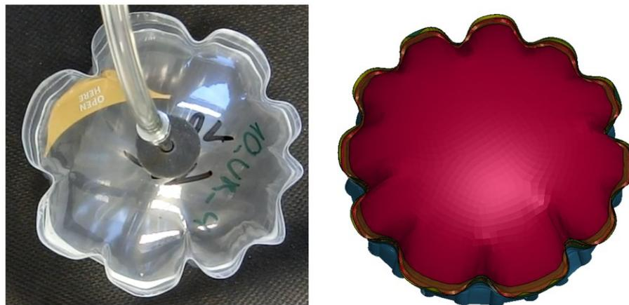
**Figure 18: Validation of the simulation results regarding the deformation of a round package with a oPA/PP peel top film sealed against a PP bottomweb at  $T_{\text{seal}} = 165 \text{ }^{\circ}\text{C}$**
