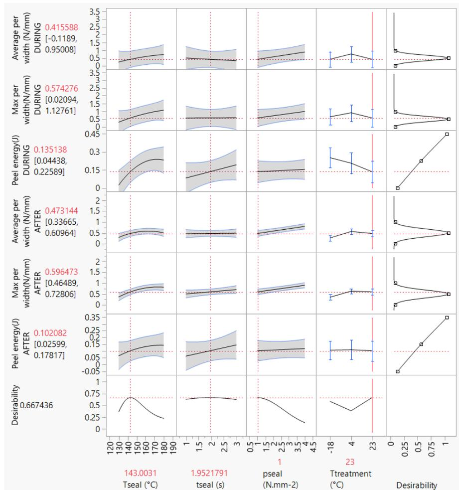
**Figure 12: Optimization (JMP®) of peel performance of PET/PE-EVOH-PE (peel) 12/45, sealed against a PET/PE bottomweb**
