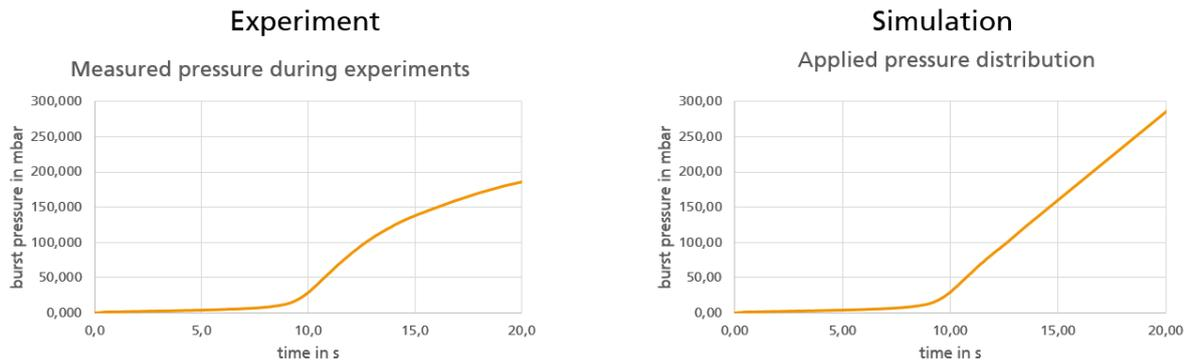
**Figure 8: Measured pressure curve recorded during burst pressure measurements (left), extrapolated pressure curve applies within the simulation (right)**
