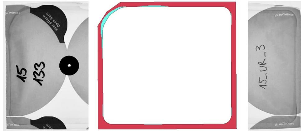
**Figure 21: Validation of the simulation results regarding the failure pattern of a cuboid package with a PET/PP peel top film sealed against a PP bottomweb at  $T_{\text{seal}} = 133 \text{ }^{\circ}\text{C}$**
