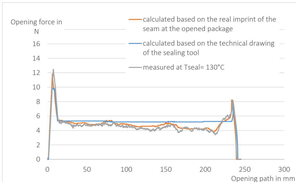
**Figure 22: Comparison of measured and calculated opening force curves of a package**
