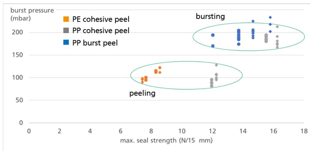
**Figure 15: Peak rupture pressure over the seal strength of the package for the three investigated peel systems**
