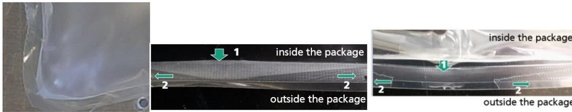
**Figure 16: Failure pattern of the sealed seal for the different peel systems and different seal strengths, PP cohesive peel at lower seal strength (left), PP cohesive peel at higher seal strength (middle), PP burst peel (right)**
