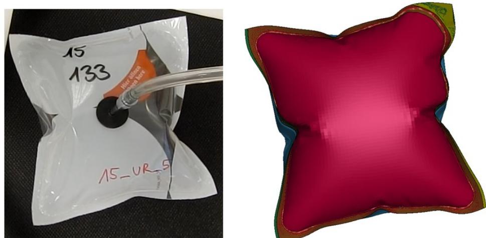
**Figure 19: Validation of the simulation results regarding the deformation of a cuboid package with a PET/PP peel top film sealed against a PP bottomweb at  $T_{\text{seal}} = 133 \text{ } ^\circ\text{C}$**
