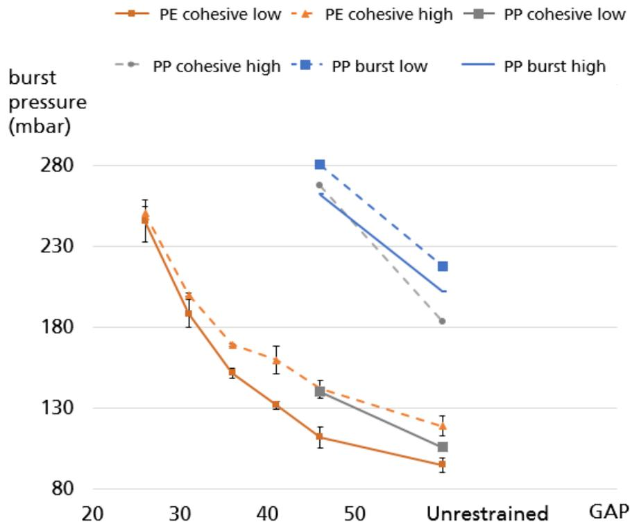
**Figure 17: Peak rupture pressure dependent on the gap between the plates for the investigated peel systems**
