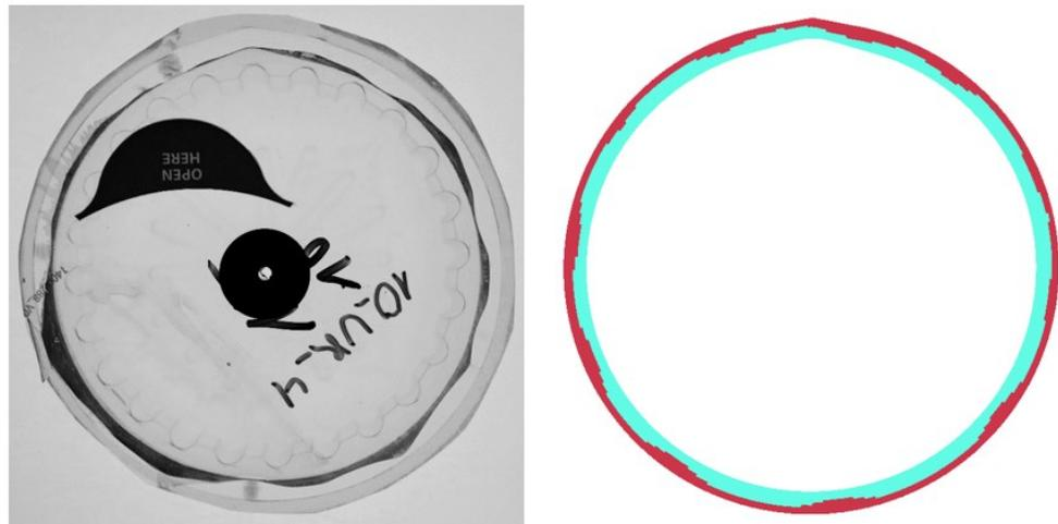
**Figure 20: Validation of the simulation results regarding the failure pattern of a round package with a oPA/PP peel top film sealed against a PP bottomweb at  $T_{\text{seal}} = 165 \text{ } ^\circ\text{C}$**
