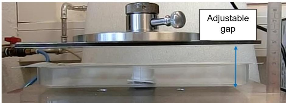
**Figure 6: Test rig for conducting burst pressure tests with adjustable gap between the plates**
