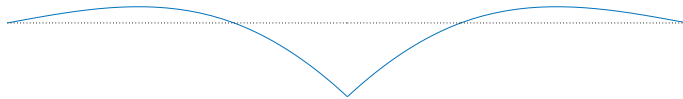
FIGURE 9 Influence line for the bending moment at midspan of a three-span beam.
