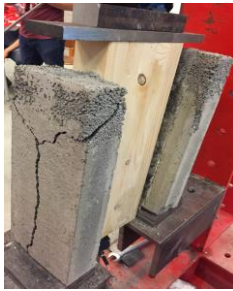
Figure 6 Failure of specimens with screws installed at 90 degrees to the timber grain
