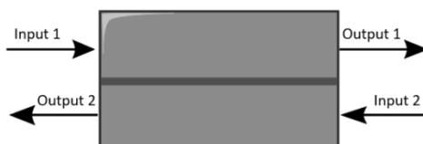
Figure 4: A schematic representation of the top view of the device, where in- and output 1 (containing the micelle solution) are separated by the membrane from in- and output 2 (containing water)
