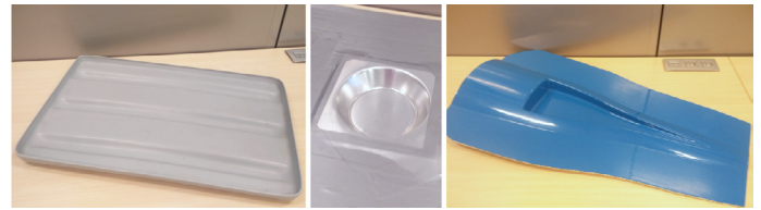
Fig. 5: Three characteristic test moulds. Left: MDPE lid with reinforcement ribs, middle: aluminium conical bowl, right: composite air grabber.
