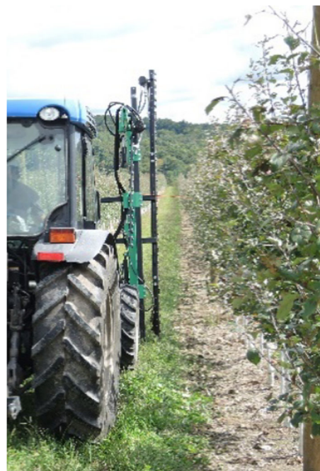
FIGURE 4 Example of a nonselective hedging system with a vertical hedging bar that trims the branches at the same distance from the trunk (He & Schupp, 2018) [Color figure can be viewed at wileyonlinelibrary.com ]
