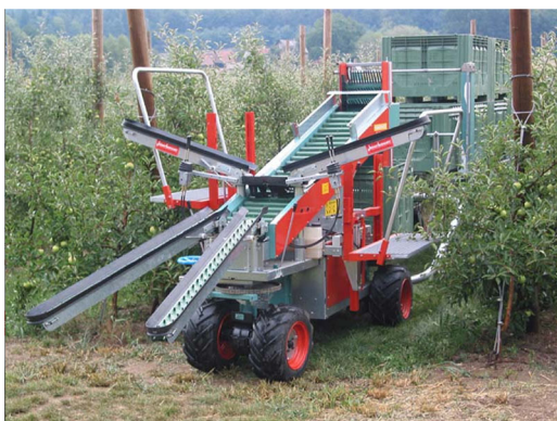
FIGURE 8 The Pluk-O-Trak from the company Munckhof as an example of an orchard aiding platform (Pluk-O-Trak; Munckhof, 2019) [Color figure can be viewed at wileyonlinelibrary.com ]
