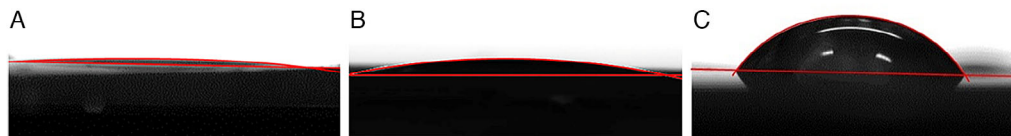
Figure 9. A) Untreated PMMA substrate with droplet of NOA89 (lens material) wetting the surface; B) substrate modified with silane APTES; C) using FOTCS as silane (see Table 3).
