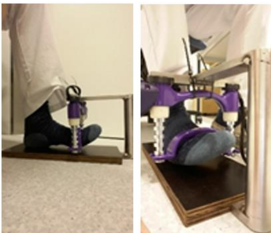
Figure 4: Datalink system to measure lower limb strength (CHU Liège).
