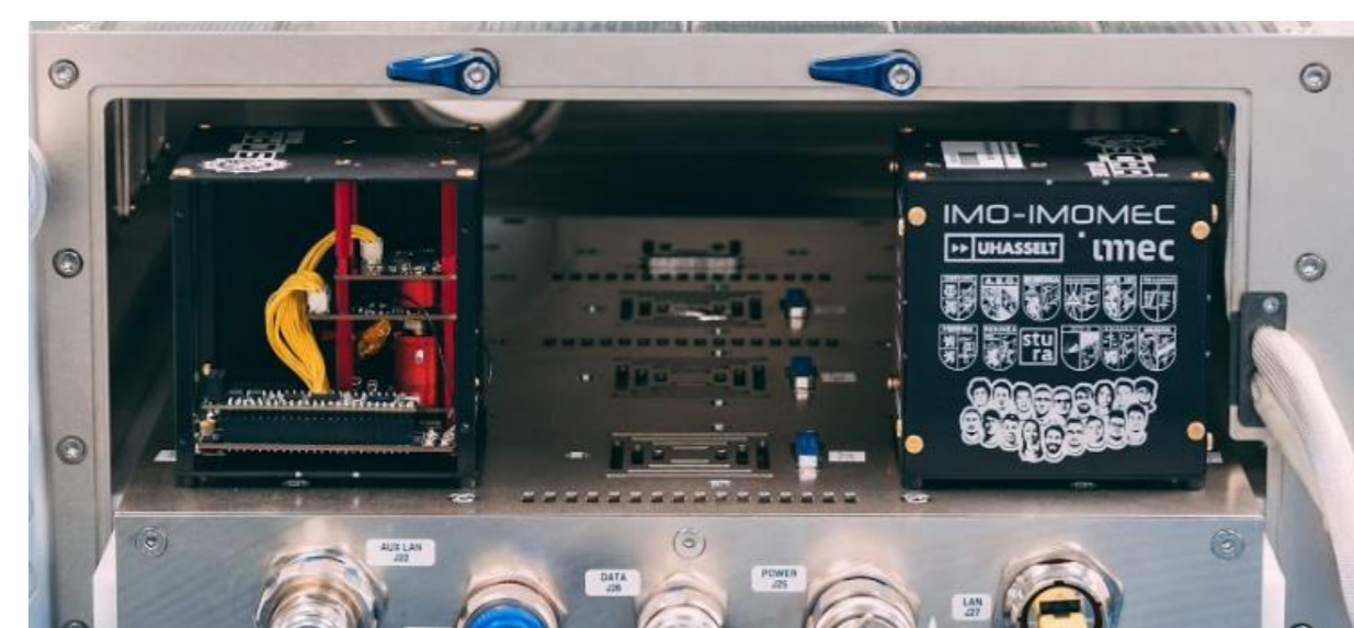
Figure 7: OSCAR-QUBE mounted on ground copy of ICE Cubes Facility
