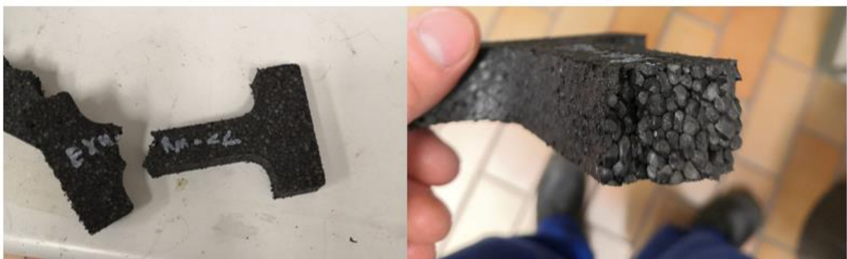
Figure 27: Sample remains after the tensile test
