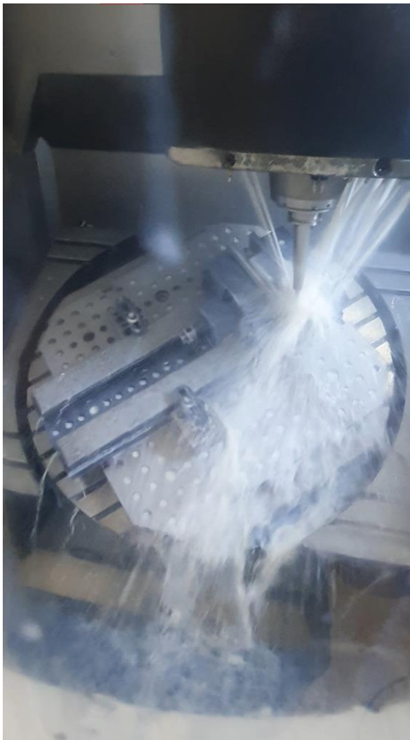
Figure 52: The 6-axis CNC-milling machine is milling the mould by repositioning the clamped object
