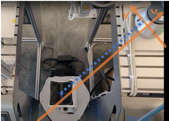
Figure 32 X and Y coordinate detection of packs
