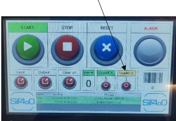
Figure 38 New HMI with 1 pack left in loader 2
