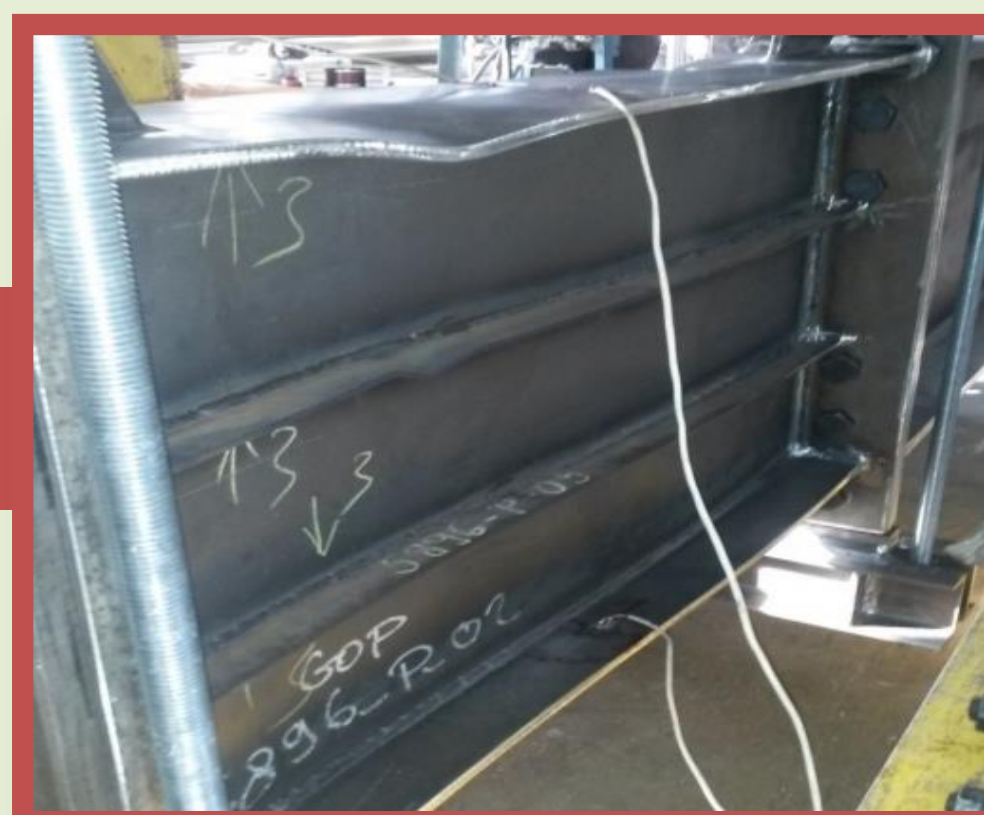
Fig. 2: Girder with two weak open-section longitudinal stiffeners
