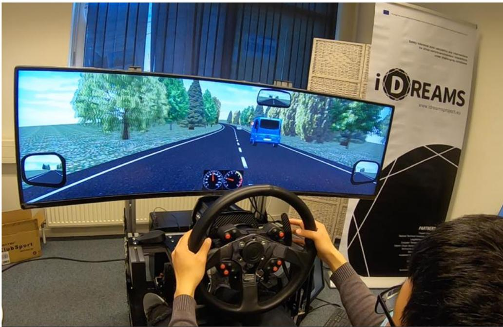
The driving simulator experiment in our study was conducted at Transportation Research Institute (IMOB) of Hasselt University. The fixed-base driving simulator was equipped with a steering wheel, an accelerator pedal and a brake pedal. The driving scene was shown on one screen as presented in Figure 3.1. The driving scenarios were designed to allow the driver overtake on a two-lane rural road with the presence of oncoming traffic on the opposing lane.
